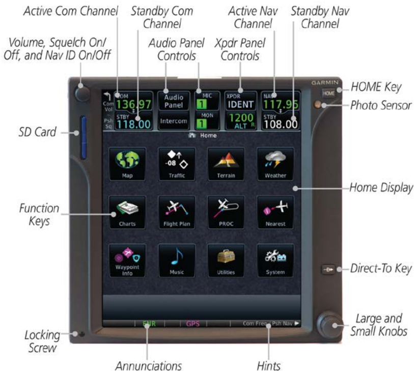
Figure 1 - GTN 750 Control and Display Layout
