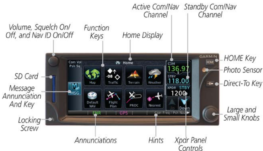
Figure 2 - GTN 635/650 Control and Display Layout
